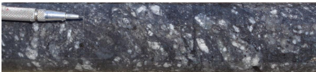
Figure 7-6: Photograph of paragneiss unit unit (From KNDD0001: 245 m)
